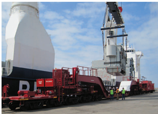
A 388-ton electrical transformer arrived on the ship M/V BELUGA RECOGNITION from Cordoba, Spain and was transloaded at the Port of Indiana-Burns Harbor onto the largest railcar ever to enter the facility.
