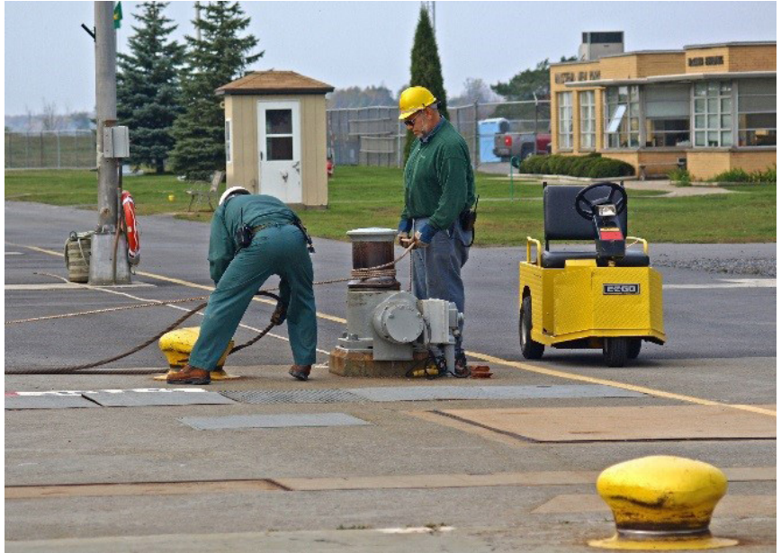
Traditional wire rope linehandling at Seaway locks.
