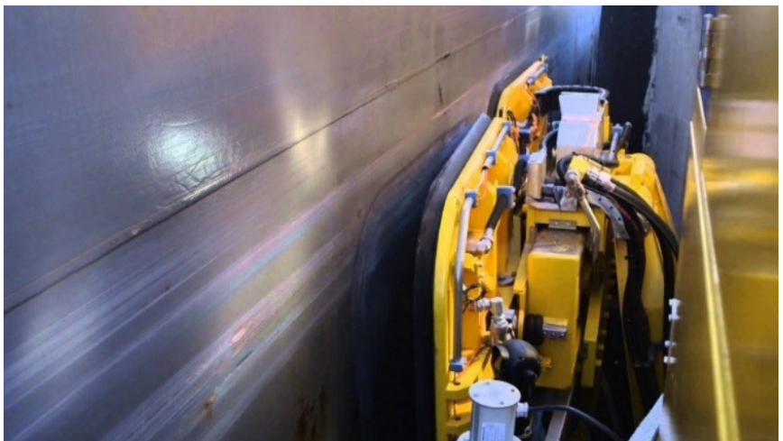
Hands-free mooring vacuum pads attached to sides of vessels for safe and efficient lock transits.
