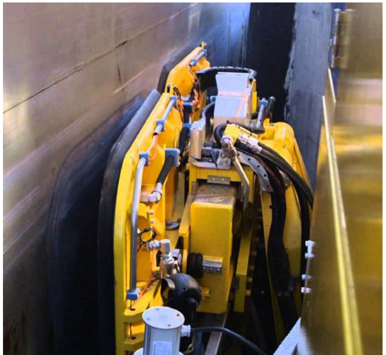
Hands-free mooring vacuum pads attached to sides of vessels for safe and efficient lock transits
