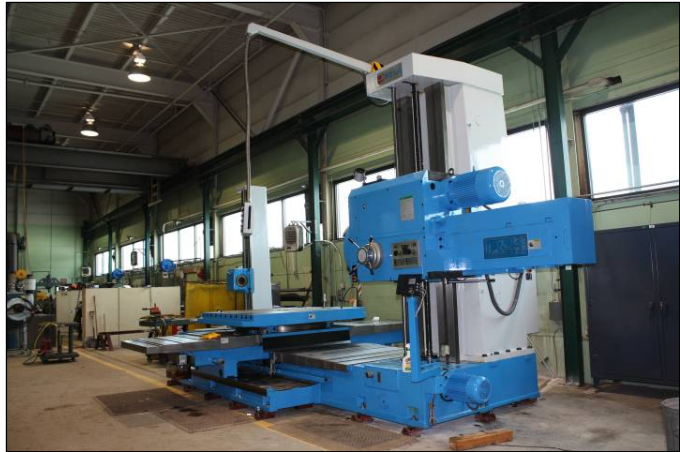
SLSDC's new horizontal boring mill to be used to repair and rebuild lock operating machinery components.
