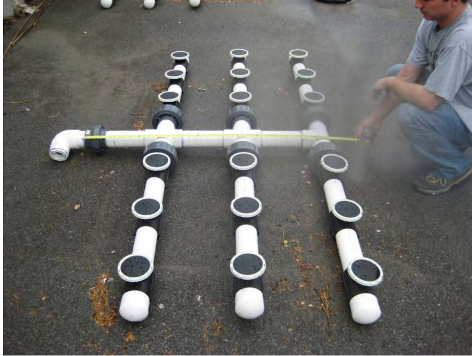
Figure 14 – Diffuser Grid of 18 Course Bubble Puck Diffusers
