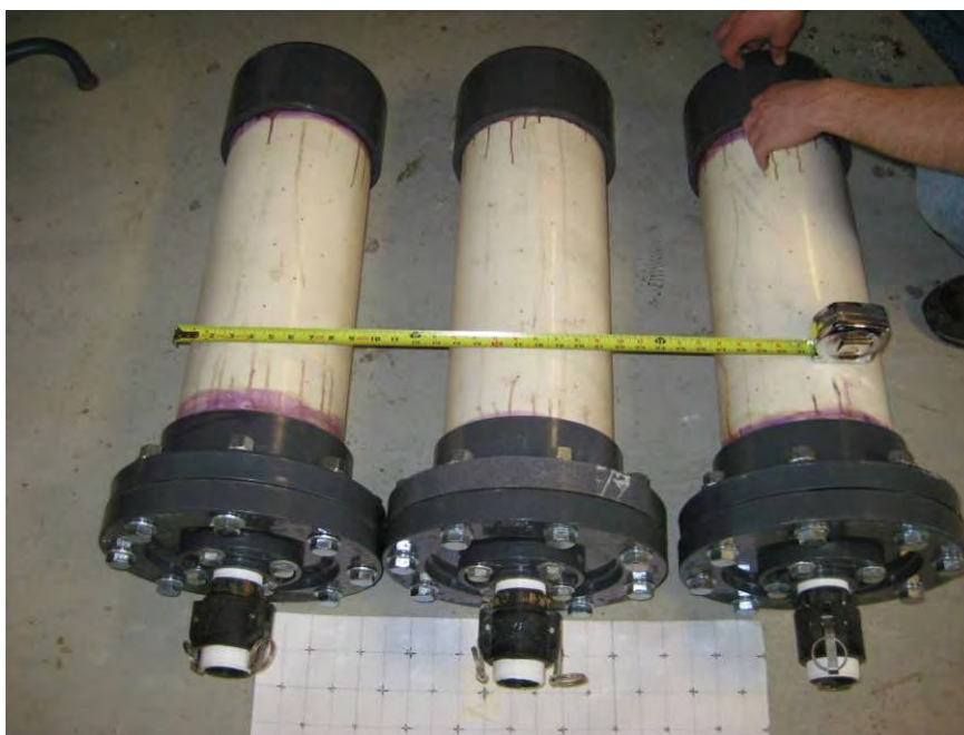
Figure 13 - Point Diffusers, 10" diameter pipes 36" long with ~100 1/8" holes
