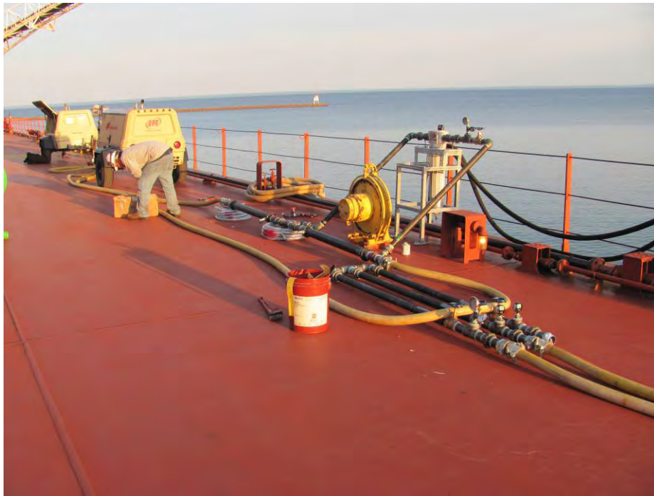
Figure 15 – Air Supply Equipment on Deck for Point Diffuser and Grid Diffuser Trials
