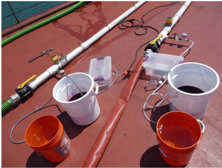
Figure 12 - Nozzle equipment on deck: hoses, valves, meters, chemical injection equipment
