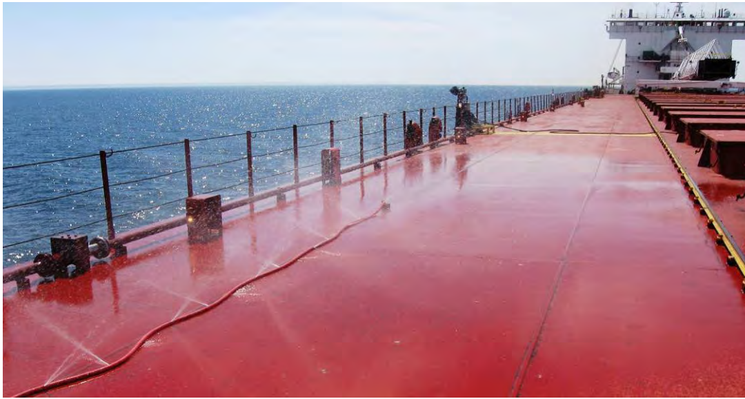
Figure 8 - Testing the Spray Pattern of the Perforated Hose
